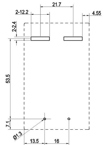
Remark:(1)In case of no tolerance shown in outline dimension:outline dimension $\leq 1$ mm,tolerance should be $\pm 0.2$ mm;outline dimension  $> 1$ mm and  $< 5$ mm,tolerance should be  $\pm 0.3$ mm;outline dimension $\geq 5$ mm,tolerance should be  $\pm 0.5$ mm.
